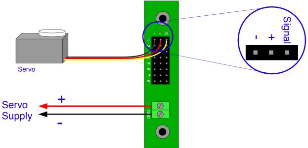
Figure 8 – Servo Outputs
