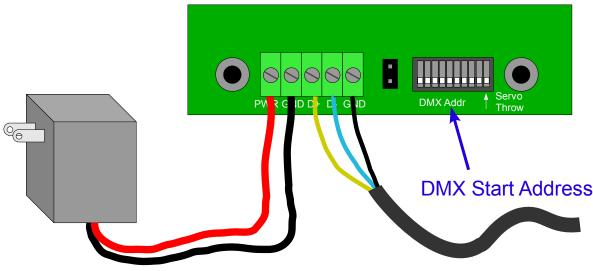
Figure 5 – DMX start address switches (1-9)
