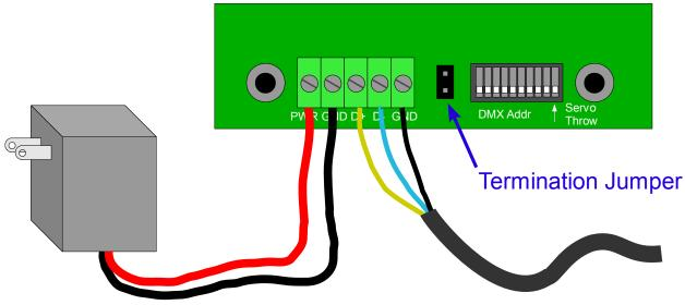
Figure 4 – Termination Jumper
